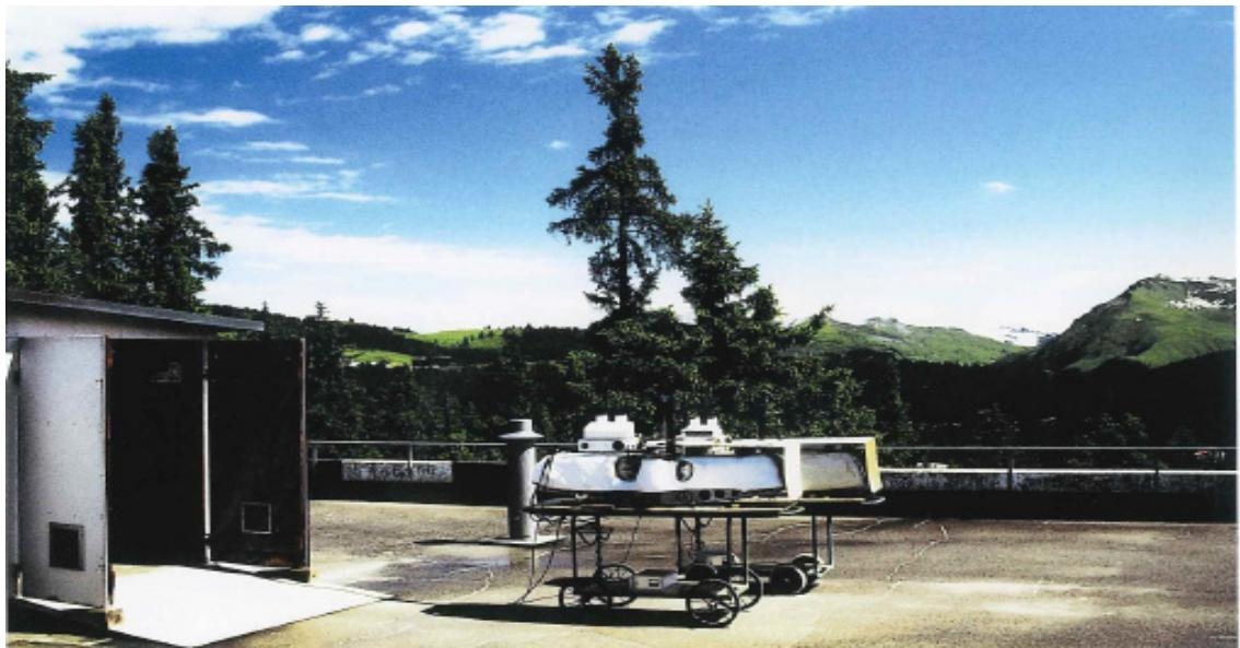
**Figure 36:** Two Dobson instruments as operated at the Haus Steinbruch before the renewal in 1987-1989. The instruments were located on trolleys enabling transport to the huts (left), where the instruments stayed during night and in case of precipitation. (Photo Kurt Aeschbacher).
