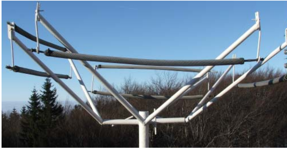
Figure A. 21 Hungarian instrument for manual icing measurement on samples of bare conductors.
