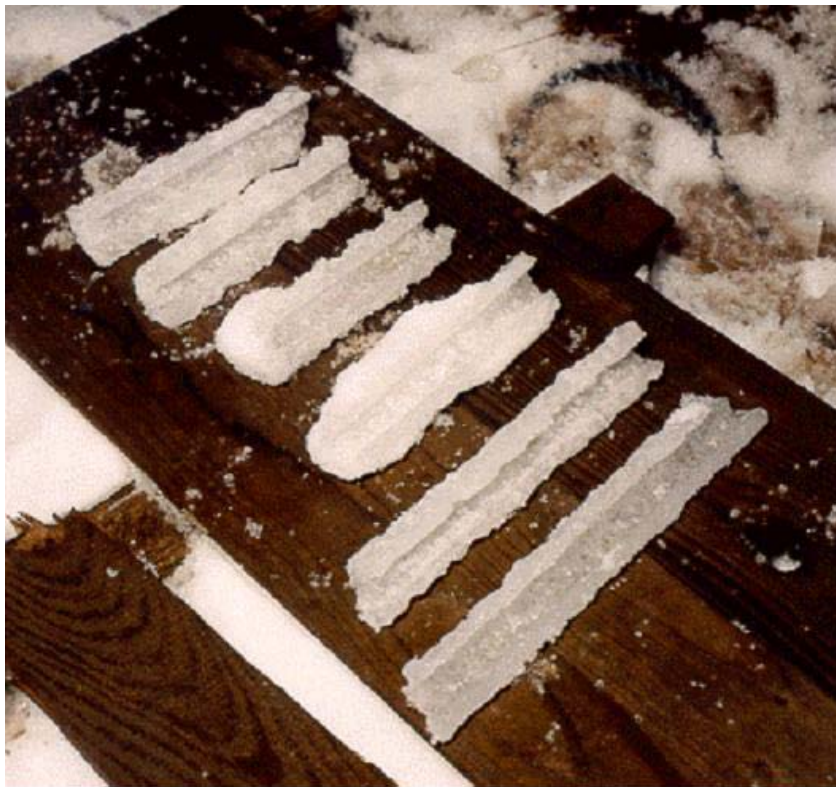
Figure A. 17 Typical accreted ice loads on different conductors after a blizzard at Deadwater Fell
