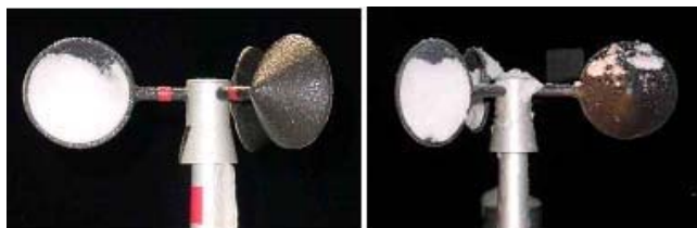
Figure A. 55 Comparison of snow deposit between wind tunnel test and field test
