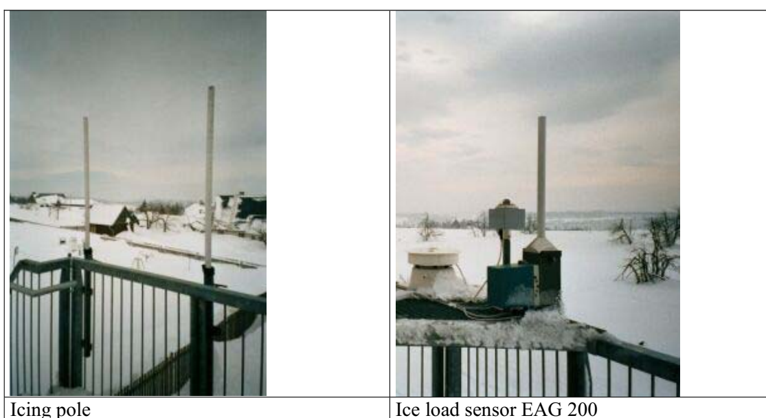
Figure A. 27 Icing measurement instruments used by German Weather Service ([37], pictures were taken at Zinnwald, February 2005)
