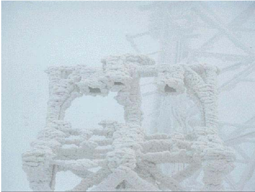
Figure A. 14 The rotating rig with snow accretion.
