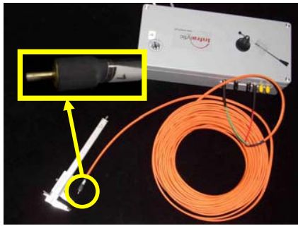
Figure A. 61 Ice detector tested
